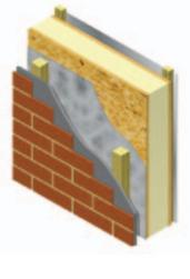
given thickness, insulation levels that can be achieved are high in comparison with other systems and masonry construction. In addition to this, the insulation and structure are effectively part of the same component so that the walls to SIP houses are relatively thin, freeing up more space for use in the rooms of the house — a factor that could be important on a small site.
